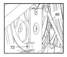
shields; there are three sizes of screws in the shields—note which size of screw you remove from each hole. Then, gently pry the shields away from the frame.
